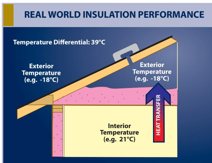
Another major flaw of the hot box approach for calculating R-Values is that it only considers one method of heat transfer: conduction. That involves heat transferred directly within a material, or between two materials that are in contact.
