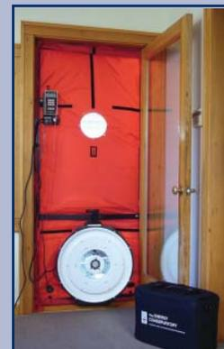
While it is true that new homes are being built more and more airtight nowadays, non-traditional insulation materials provide giant leaps in tightness, minimizing seams and gaps, and consequently air leakage. Homes constructed with structural insulated panels regularly achieve air tightness levels of 1 to 2 ACH @ 50 PA. These impressive results contribute directly to real world energy efficiency improvements.
